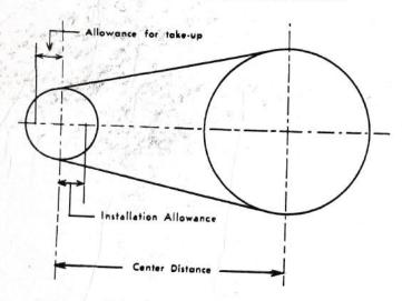
Due to variations in Belt Lengths and Pulley Diameters the Center Distance shown in Table VI may vary. For this reason it is good practice to make a trial installation
