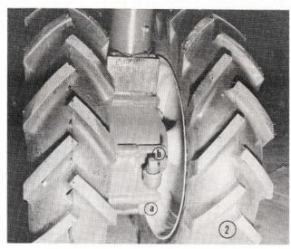
on an 8-hour day). The Ring Gear Assembly has an Oil Level Plug (a) and an Oil Filler Plug (b). When oil is at the proper level, it should be level with opening when plug (a) is removed. To check, open plug (a) and if the lubricant is not to this level, add lubricant through Oil Filler Plug (b) until it begins to run out plug (a). Use Mobiloil 140.
