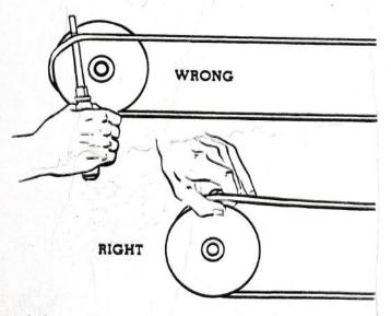
before setting your permanent Center Distances. Prying or forcing may damage belts internally and reduce life. When proper provision is made for installation, belt can be laid in groove as shown.
