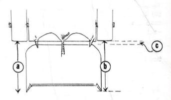
Note that the Mower Unit MUST BE A-LIGNED with the main unit of the machine for the blades to cut correctly. Make certain that the space between the front of the right-hand traction wheel and the right-hand front of the Mower Unit (a) is the same as the space between the left-hand traction wheel and the left-hand front of the Mower Unit (b). Unless the lines formed by the rear edge of the Mower Unit and the front edge of the unit are parallel (c), the blades may skip and cut unevenly.
